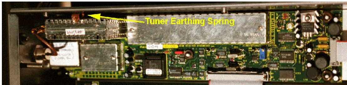
Picture 21 - COFDM Tuner Earthing - Original State
